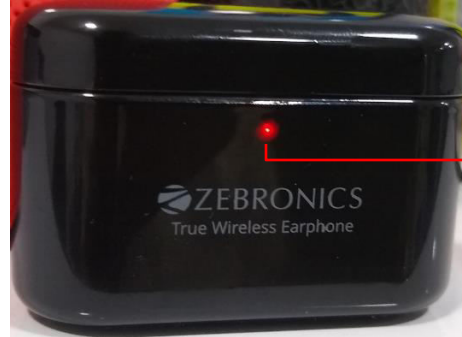
Charging Indicator for Case Red LED Blinks: Charging Indication RED LED Glows: Full Charging Indication
