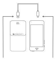
Output Port USB / Type C x 2 Device with Type-C / Micro USB Lightning Support • Connect the Type C/USB end of the charging cable to the device and the USB/Type C end to the output ports of the power bank.
