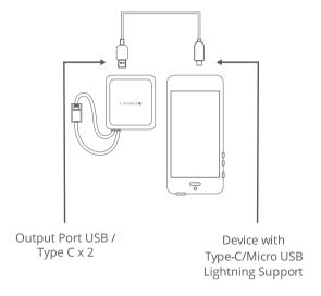
Connect the Type C/USB end of the charging cable to the device and the USB/Type C end to the output ports of the power bank.
