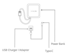
Connect the Type C end of the charging cable to the power bank and the USB end to the charger. Or can charge through Built in USB cable.
