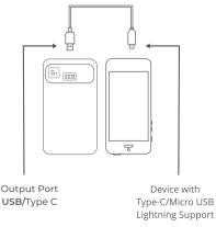
Connect your device with the Type C connector or Micro USB connector end of the cable and connect the other end of the cable to the power bank output port.
