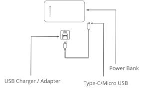
Connect the Type C/micro USB end of the charging cable to the power bank and the USB end to the charger / adapter with a DC 5V output.
