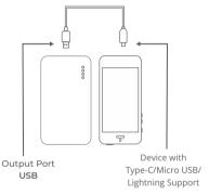
Connect your device with the Type C connector /micro USB connector or lightning end of the cable and connect the other end of the cable to the power bank USB output port.
