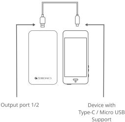
Connect your device with the Type C connector or Micro USB connector end of the cable and connect the other end of the cable to the power bank.
