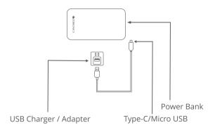
Please charge the power Bank with rated (DC 5V/3A, DC 9V/2A, DC 12V/1.5A) with Type C power Adapter and DC 5V/2A, DC 9V/2A, DC 12V/1.5A with Micro USB power adapter.
