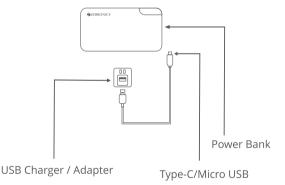
Connect the Type C/micro USB end of the charging cable to the power bank and the USB end to the charger / adapter with a DC 5V output.
