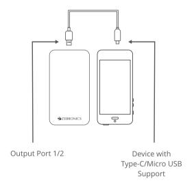
• Connect the Type C/micro USB end of the charging cable to the device and the USB end to the output ports of power bank.
