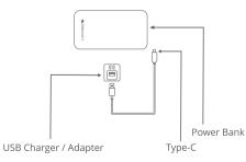
Connect the Type C end of the charging cable to the power bank and the USB end to the charger or adapter with a Type C (DC 5V/3A, DC 9V/2A, DC 12V/1.5A) cable.
