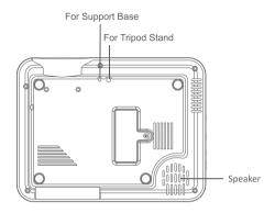
**Note:** The adjustable support base can assure the max projection angle by 15°, The best display effect will be obtained by projection angle ranges of  $0^{\circ}$  -  $8^{\circ}$ .
