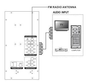
**Note:** Insert the plugs fully into the jacks. Loose connections may produce noise interference.
