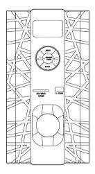
**INPUT**: Input function key. **5.1/2.1**: 5.1/2.1 function key.
