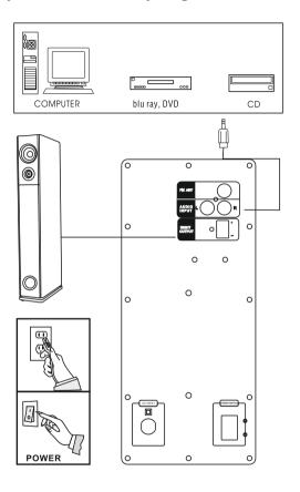
**Note:** Insert the plugs fully into the jacks. Loose connections may produce a humming sound or other noise interference.
