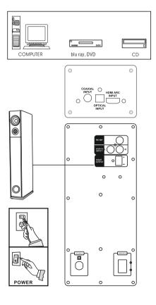
**Note:** Insert the plugs fully into the jacks. Loose connections may produce a humming sound or other noise interference.
