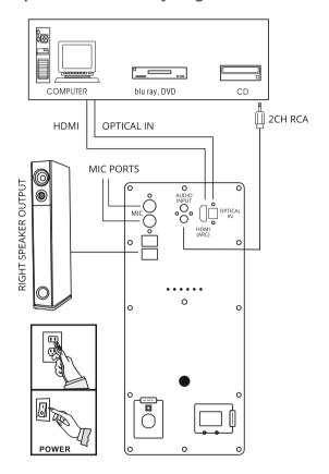
**Note:** Insert the plugs fully into the jacks. Loose connections may produce a humming sound or other noise interference.
