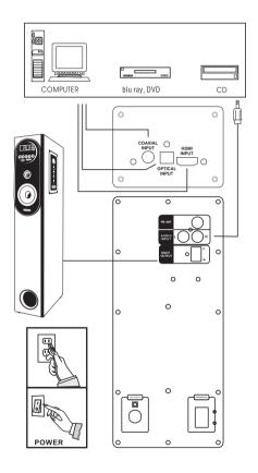
**Note:** Insert the plugs fully into the jacks. Loose connections may produce a humming sound or other noise interference.
