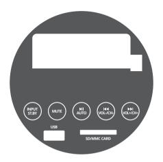
VOL- / CH- | MOVES to the previous track for play if in USB or SD or BT Mode moves to the previous channel if in the FM Mode / Decreases the volume level if touch and hold continuously.
