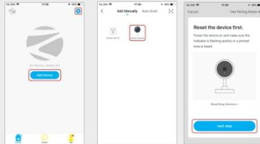
Select your WiFi "SSID", enter corresponding "password" and tap next, the Mobile prompts a QR Code, hold the camera 15-20 cm in front of the Mobile Phone to scan the QR code.
