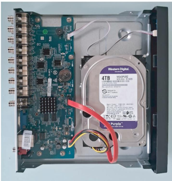
3. Secure the hard disk to the hard disk screw holes on the baseplate.
