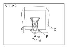
• By using the provided Allen Key, Fasten the included screws into the mounting points of the Seat Cushion as shown in the reference image.
