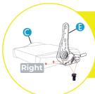
Remove the pre-installed 2 no of screws. Align seat C and adjuster E with seat holes, and tighten the screws as shown in image.
