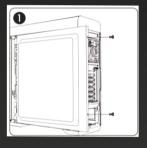
Undo the thumb screws and remove the cabinet side panel.
