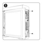
Undo the thumb screws and remove the cabinet side panel.
