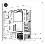
Fasten the power supply in the cabinet with provided screws.
