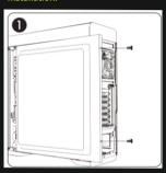
Undo the thumb screws and remove the cabinet side panel.
