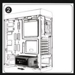
Install the power supply inside the cabinet.
