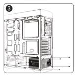
Fasten the power supply in the cabinet with provide screws.
