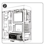
Install the power supply inside the cabinet.
