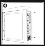
Fix back the cabinet side panel and fasten the thumb screws.
