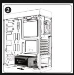
Install the power supply inside the cabinet.
