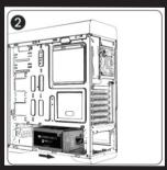
Install the power supply inside the cabinet.
